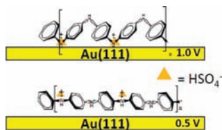
Figure 3. Schematic presentation of the relative positions of polyaniline and coadsorbed bisulfate ion on Au(111) prepared at 1.0 and 0.5 V.
